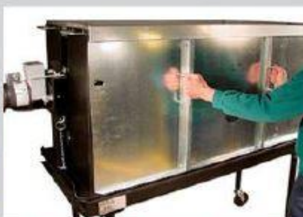
5. Place Front Panels in place after starting fire.
